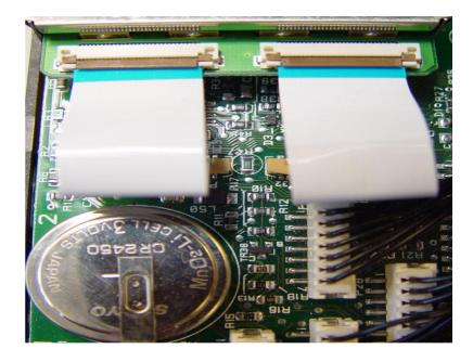
PCB87 has to be replaced with PCB85 (part no: 8000766) in products between the serial nos. 14923175 and 15955832.
